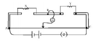
When a resistance of  $15\Omega$  is connected in series with 'Y', the null point is found to shift by 10cm towards the end A of the wire. Find the position of null point if a resistance of  $3\Omega$  were connected in parallel with 'Y'.
